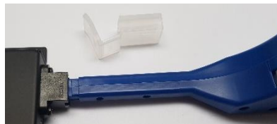
Cleaning tool with adaptor removed and the tip in a through adaptor for cleaning internal connector or a Fibre port requiring cleaning
